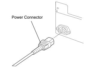
**3.** Plug the other end of the Power Cord into a grounded outlet as shown in the figure below.
